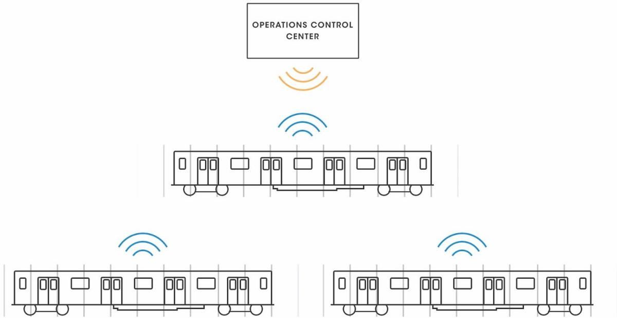
Through a wireless communications network, MTA trains and tracks will share individual sensor data with the operations control center.
